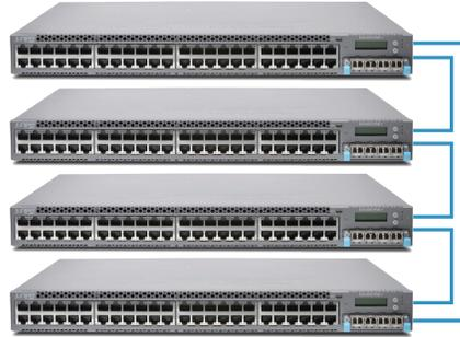
Figure 1: Virtual Chassis configuration
