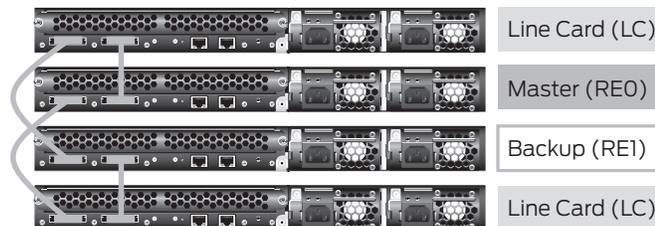
Figure 6: Recommended member location in a braided-ring deployment
